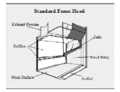
a. **Airfoil.** Found along the bottom and side edges, airfoils streamline airflow into the hood preventing the creation of turbulent eddies that can carry vapors out of the hood. The space below the bottom airfoil provides a source of room air for the hood to exhaust when the sash is fully closed.
