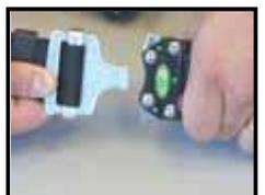
**Quick-Connect Buckles** – Inspect the buckle for distortion. The outer bars and center bars must be straight. Make sure dual-tab release mechanism is free of debris and engages properly.
