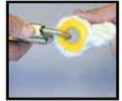
**Wire Rope Lanyard** – While rotating the wire rope lanyard, watch for cuts, frayed areas, or unusual wearing patterns on the wire. Broken strands will separate from the body of the lanyard.
