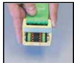
**Friction and Mating Buckles** – Inspect the buckle for distortion. The outer bars and center bars must be straight. Pay special attention to corners and attachment points at the center bar.
