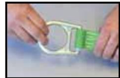
**Attachment of Buckles** – Inspect for any unusual wear, frayed or cut fibers, or broken stitching of the buckle or D-ring attachments.
