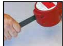
Check the hardware as directed above. The snap hook load indicator is located in the swivel of the snap hook. The swivel eye will elongate and expose a red area when subjected to fall arresting forces. Do not use the unit if the load impact indicator has been activated.
